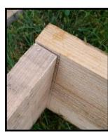
**STEP 4: Build the frame.** Using the star driver bit use the pilot holes as a guide to screw the boards together with the 2.5 inch screws in three places: top, middle, and bottom. Repeat at the remaining 3 corners. Do not attach the cross bracing board yet.
